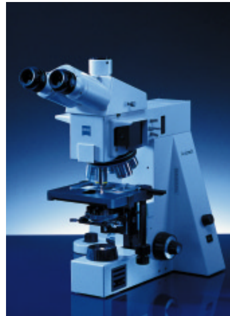
Axiotech for reflected and transmitted light methods (reflected light 30-watt, transmitted light 30-watt halogen lamp)
