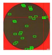
MicroView capture locations are displayed on the wafer map and ProcessGuard provides options for capture and image review.
