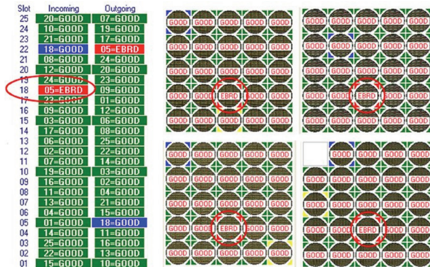
Figure 3. Slot position analysis showed that the problem repeatedly affected the wafer in slot #18.
